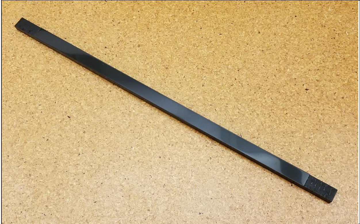
Figure 3.4 One of the polypropylene beams made using the laser cutter.
